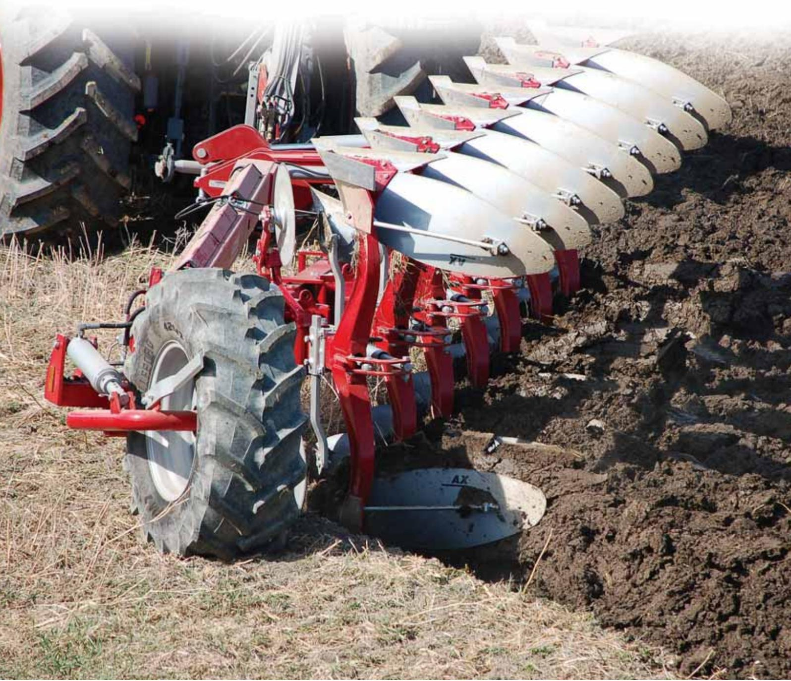
**Beamhouses:** The beamhouses on HSRWT/S are based on the same strong ones as used on the fully mounted XRWT/S. The geometry gives low forces in beam houses and cylinders. The beam houses and the other moving parts on the plough are greasable and equipped with replaceable bushings.
