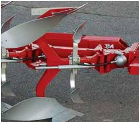
**Stone trip system:** Agrolux ploughs can be equipped with gas hydraulic stone trip system for nonstop ploughing even in tough conditions with large stones, or shear bolt protection for conditions with few fixed stones. The hydraulic system offers the opportunity to set the trip force individually for each pair of bodies. This makes it possible set the pressure higher for the front furrow in order to keep it still in the soil without exposing the plough and the tractor to higher load.
